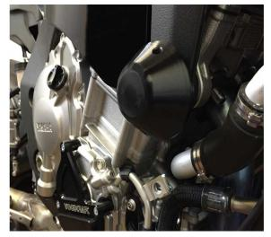
3) Slide the plastic slider over the top of the base and secure it in place using
